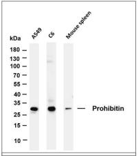
Various whole cell lysates were separated by 4-20% SDS-PAGE, and the membrane was blotted with anti-Prohibitin (ANT0004R) antibody. The HRPconjugated Goat anti-Rabbit IgG(H+L) antibody was used to detect the antibody. Lane 1: A549 Lane 2: C6 Lane 3: Mouse spleen Predicted band size:
